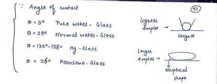
Note - 1 As the diameter of the tube reduces, the capillarity effect increases. In manometers, the diameter of the at tube are more than 10 mm to avoid the capillarity effect in pressure measurement
